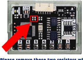
Please remove these two resistors when using the emulator on Hyundai new type steering lock.
